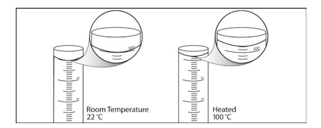
7. Using what you know about the attractions between water molecules and the way heat affects molecular motion, explain why the volume of water in the cylinder increases when it is heated.
